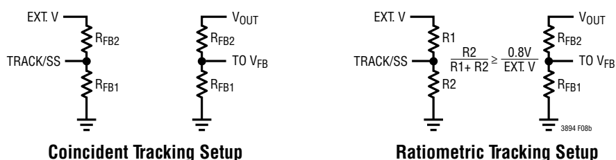
Figure 9(b): Setup for Ratiometric and Coincident Tracking
